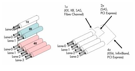
Each device bay signal connector has a 100-pin connector with 64 high-speed signal pins hard-wired from the device bay connector to the interconnect bays. This results in 16 lanes ( $64 \div 4$ ) to each interconnect bay. This provides at least two lanes to each interconnect port for connectivity to LAN, storage area network (SAN), InfiniBand, or any other interconnect type. Full-height servers occupy two half-height device bays and therefore have up to 32 lanes available.
